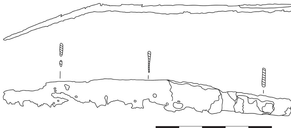
Fig. 4 The scramasax knife from Milking Pen Lane. The knife is shown viewed from the top (above) and from the left side (below). The knife is heavily corroded. Much of the blade has been lost leaving a portion with a very lacy appearance. The cross-section shape and plan in side view form a limited representation of the original blade. Traces of organic handle components may be present in mineralised form on the left side of the tang. The scale is 5 cm long
