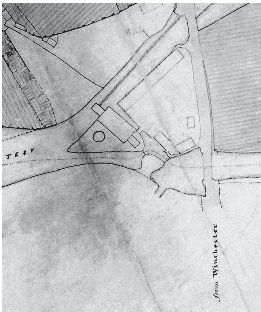
Fig. 4 Detail from the 1839 plan, surveyed in 1819. It is not completely accurate in that the mill is shown about 2m too far to the north-west
