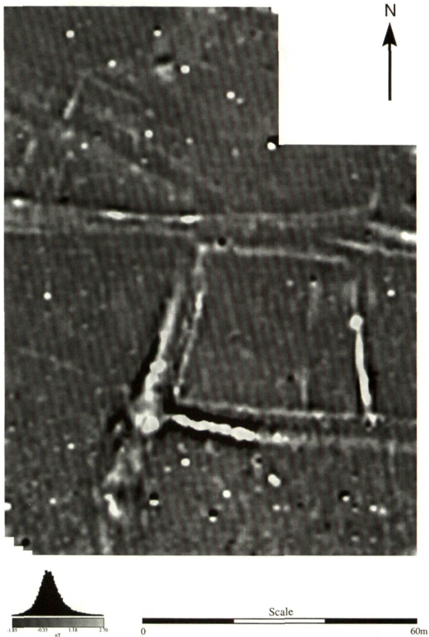
Fig. 14 Magnetometer survey of the environs of the Roman Villa (from Busby 1994, with permission). The SW sector of the survey corresponds with the excavated area (see Fig. 2)
