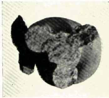
Fig. 9. SECTION OF THREE-STRAND CABLE SHAFT.
